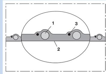
Suction and transport hose; Heavy, smooth interior, grounding wire
